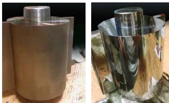
Before and After photos of an A2 component finished with 3 micron SC compound on a felt wheel
